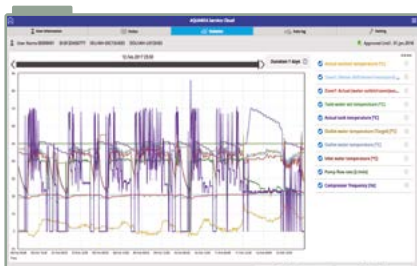
Statistics tab. Customisable statistics of a maximum of 71 parameters. Available anytime with the information of the last 7 days.
