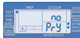
6. Heating priority (YES/NO, Standard: NO). If possible, this value should be left as NO, as otherwise hot water is only heated with the electric immersion heater.
