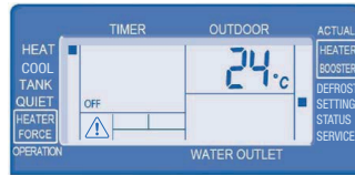
5. Target temperature for switching off heating mode (limit heating temperature, 5 to 35 °C, Std. 24 °C)
