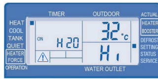
4. Water supply target temperature for heating mode at high outside temperature (25 to 55 °C, Std. 32 °C)
