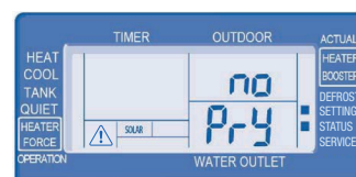
5. Solar priority (YES/NO, Standard: NO) If a solar thermal system is used, this value should always be set to YES.
