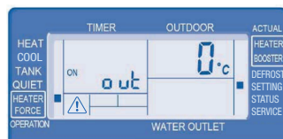
6. Outside temperature for switching on the additional electric heater (-15 to +20 °C, Std. 0 °C)
